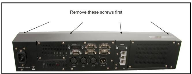
FIGURE 7. KP 32 CLD Top Screw Removal.
